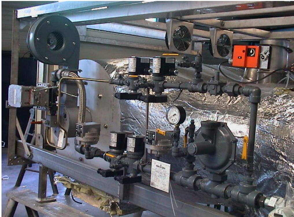
Figure 3.4 Burner + Gas line
