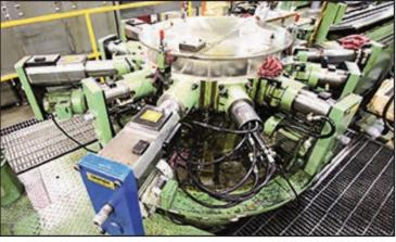
HYDROMAT HW25/12 ROTARY TRANSFER MACHINES
